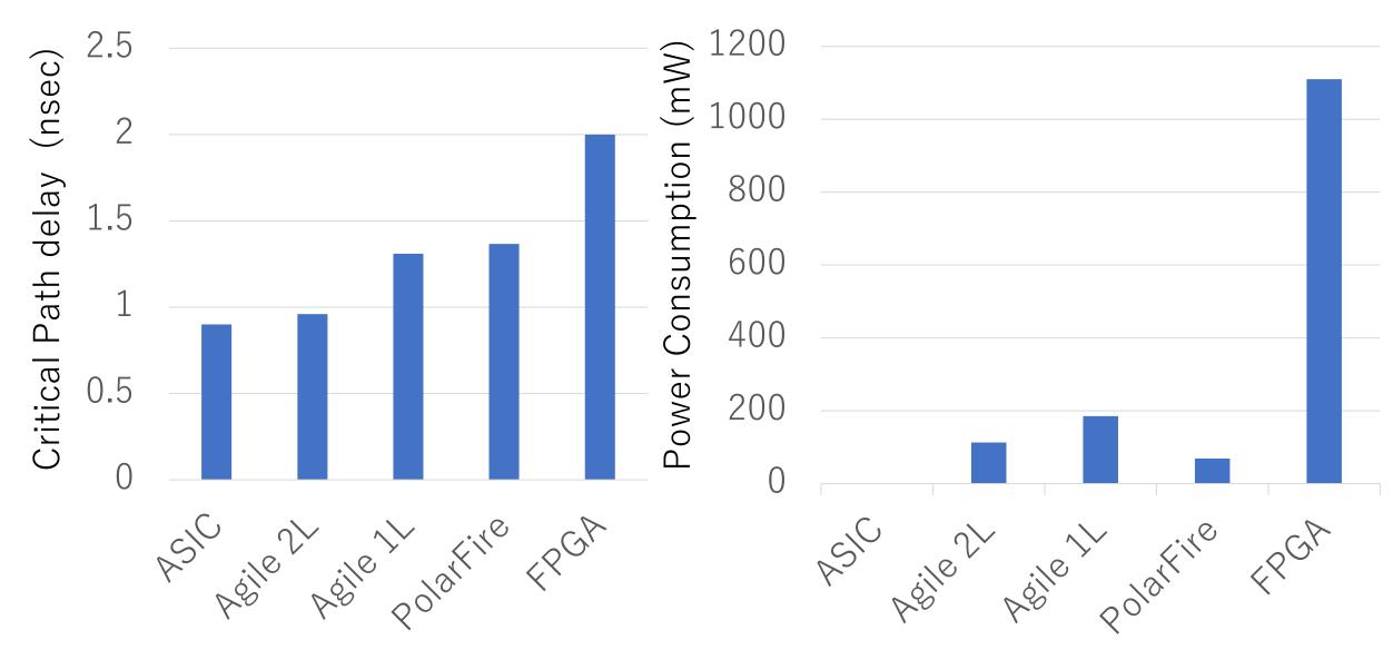
Agile 2L is better than Polarfire and SRAM FPGA in terms of performance. Polarfire appears to reduce power consumption at the expense of performance. DCT
