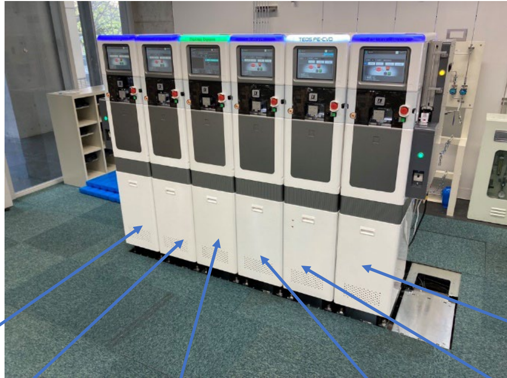
Maskless exposure, TEOS PE-CVD Development Acetone cleaner
